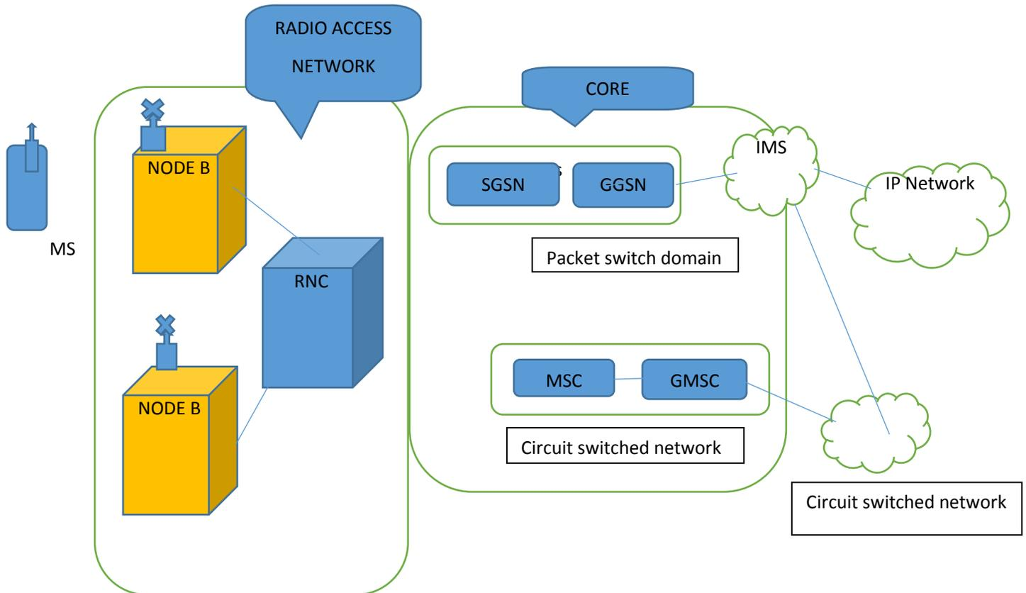
Figure 2.5 UMTS Network architecture [12]
