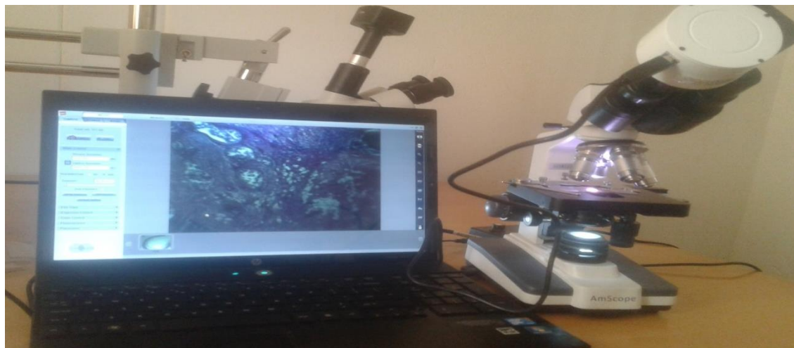
Figure 3.7. Stereo microscope (XSZ-107BN Series) linked to an HP-ProBook 4510s with ISC Capture software.
