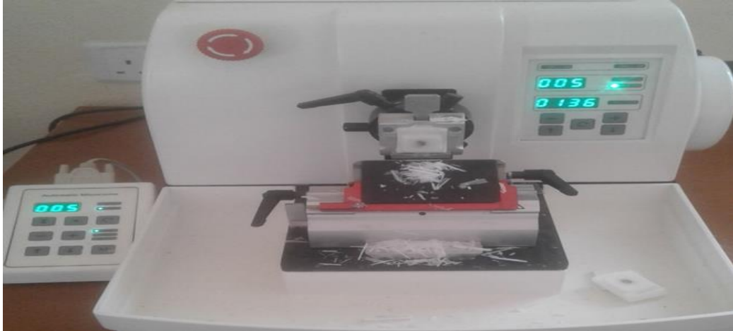
Figure 3.4. Full Automatic Microtome (ZHCHEING, CHINA) cutting a tissue block
