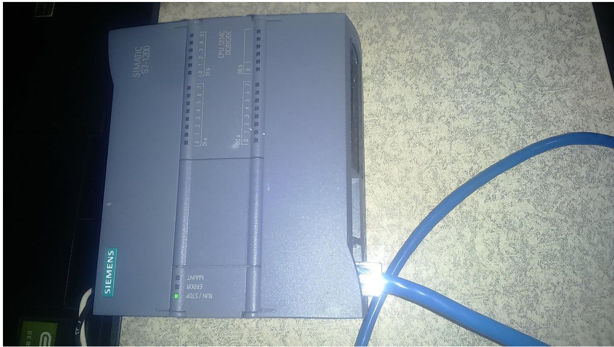
Fig 4.3 Powered S7-1200 PLC
