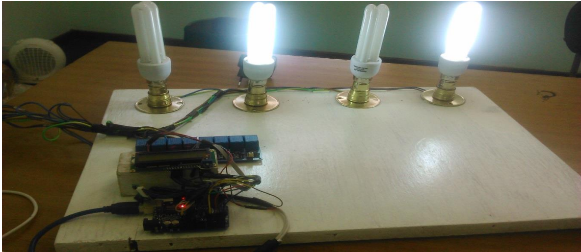
Figure 4.1: The RF home automation system working
