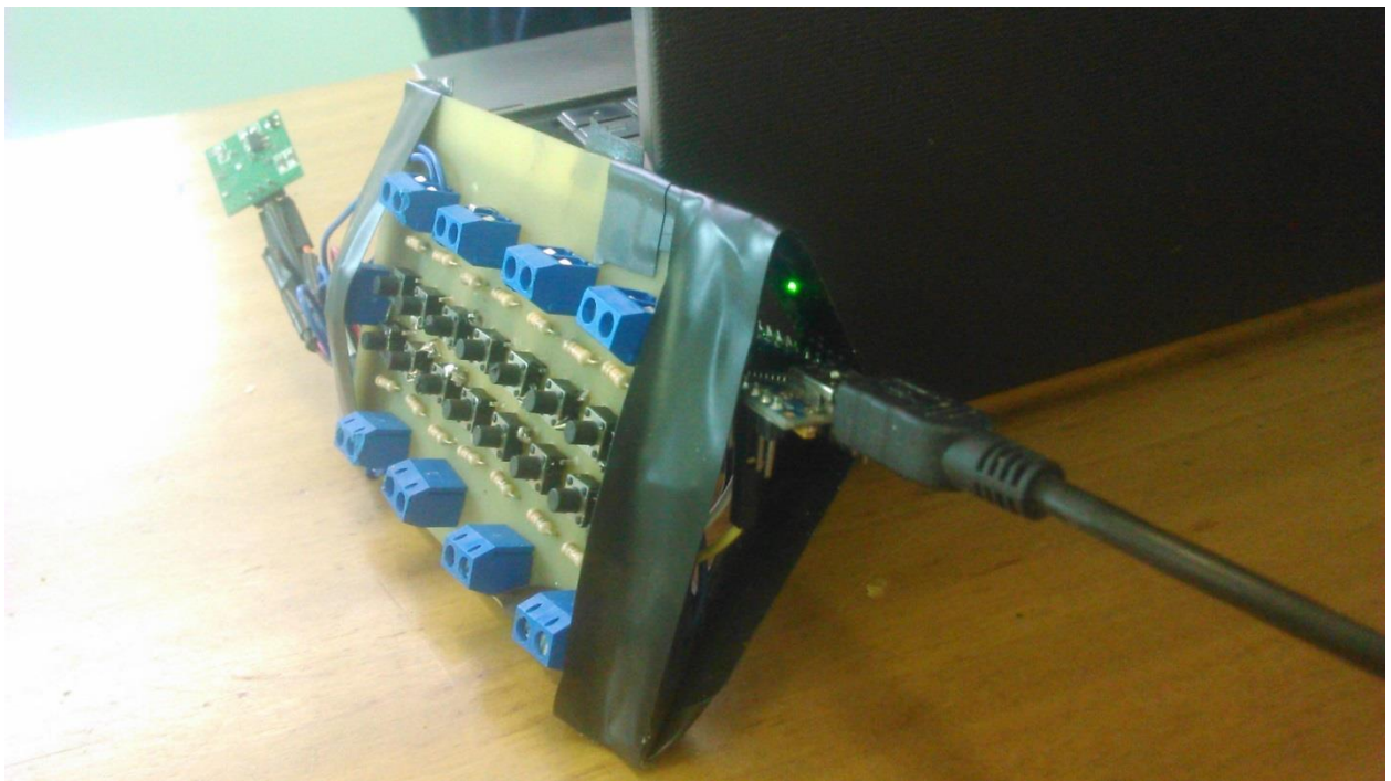
Figure 4.2: Remote controller to switch appliances ON/OFF
