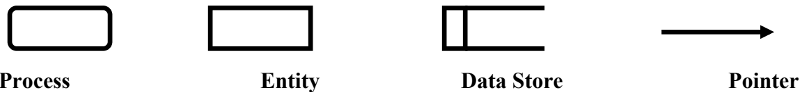
Fig 4.3: Key to dataflow diagram
