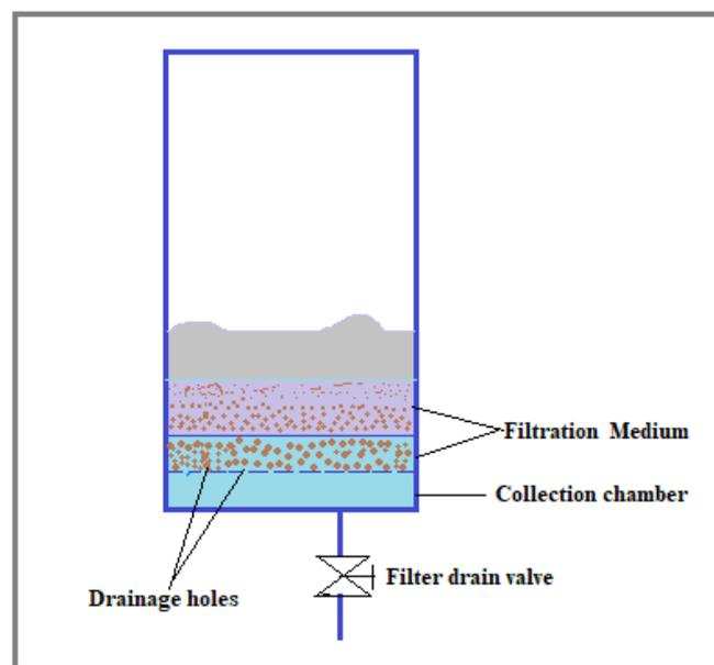
Figure 4.1 – Filter under drainage system illustration
