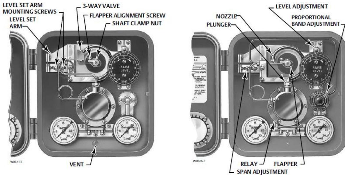
**Figure 2.10 - interior of a Pneumatic level controller [7]**
