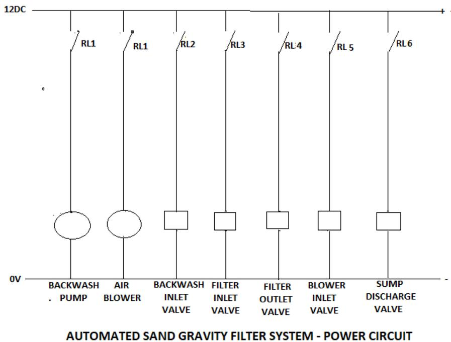
Fig 3.7 – Power circuit for the full system
