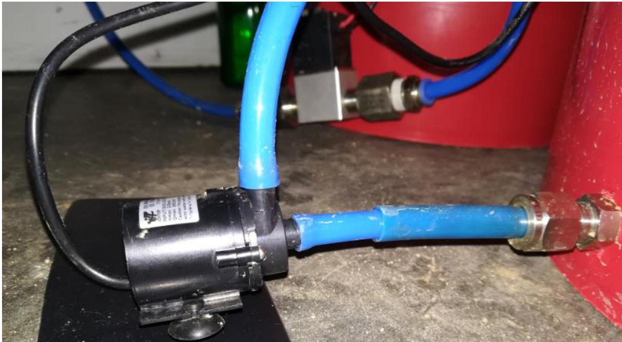
**Figure 3.4 – 12V dc Pump Mounted**
