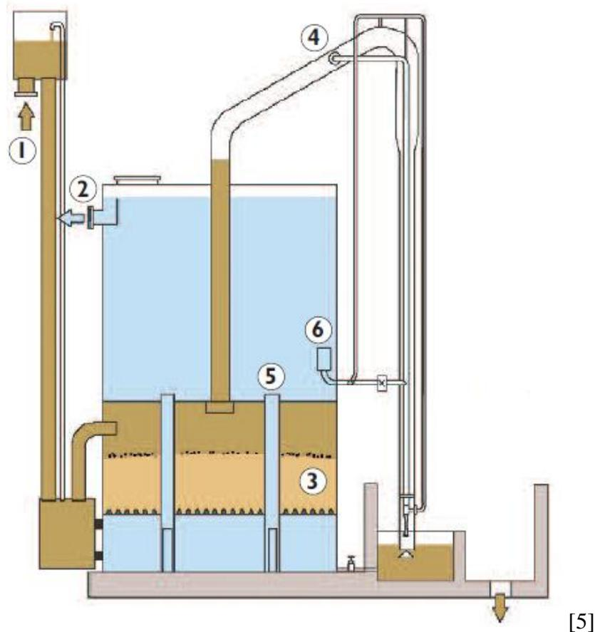
**Figure 2.5 -The Autonomous Gravity Sand Filter (AGF)**
