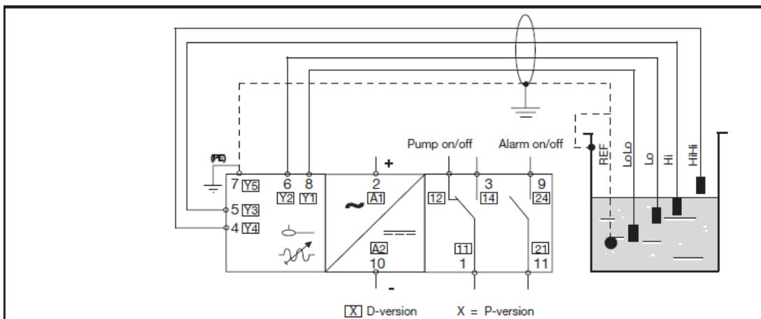
Figure 2.8 – 5 sensing probe – Level controller [6]
