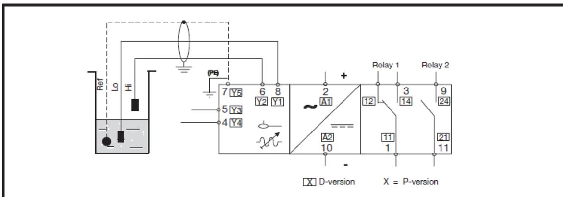
Figure 2.7 – 3 sensing probe – Level controller [6]
