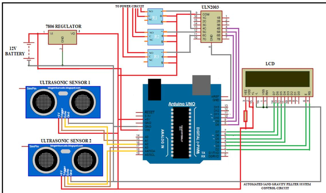
Figure 3.9 – Summarised Control circuit
