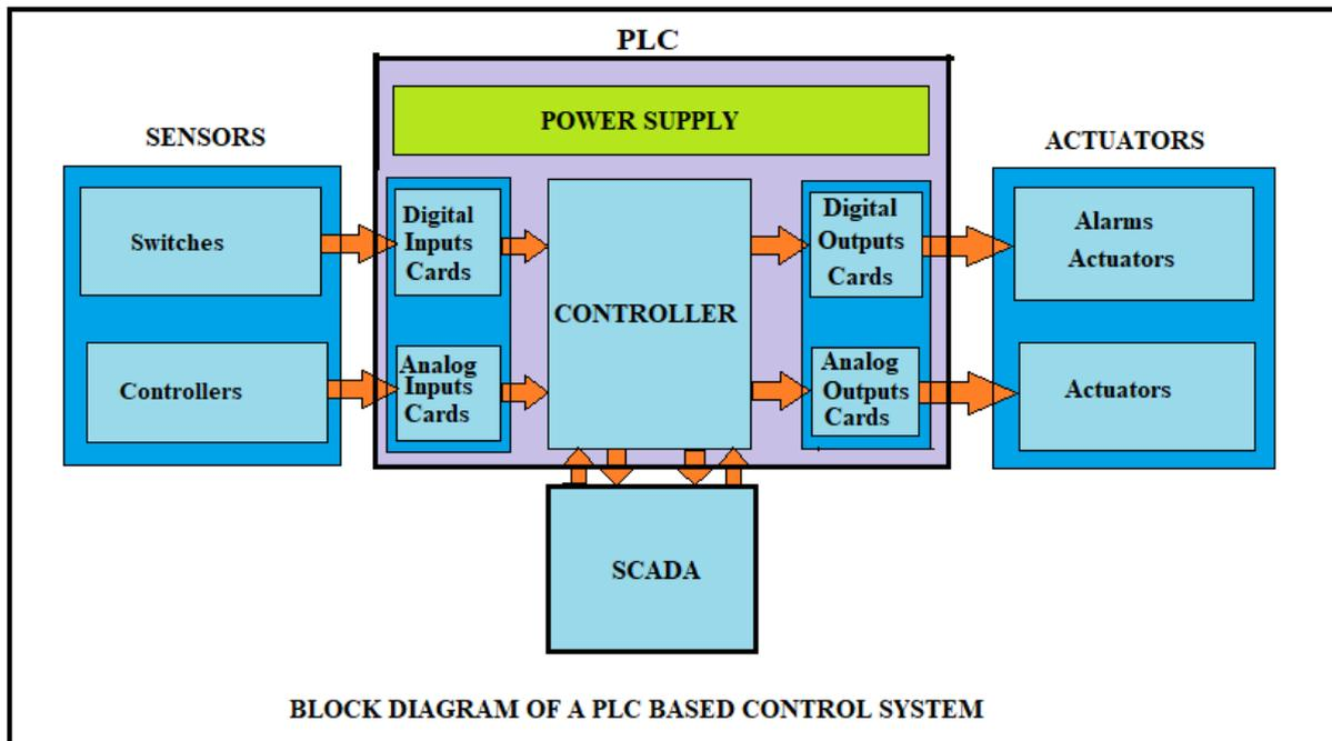
**Figure 2.12 – PLC Based control system**
