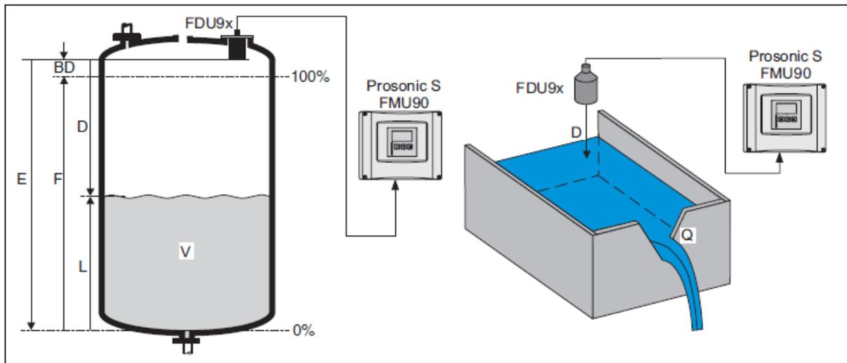
**Figure 2.11 – Prosonic level control block diagram**
