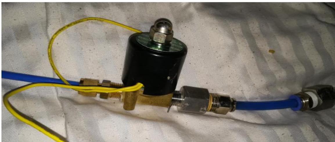
**Figure 3.3 – 12Vdc Solenoid valve with connections**
