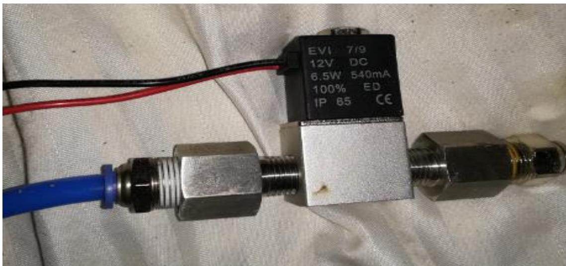
**Figure 3.2 - 12Vdc Solenoid Valve with connections**
