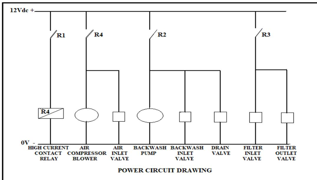
Figure 3.5 – The Power circuit diagram
