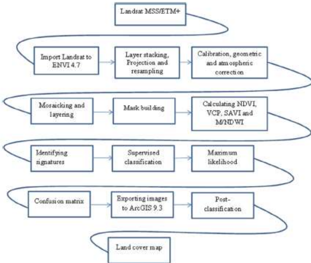
Figure 7: Generalized Landsat Image Processing in ENVI4.7 and ArcGIS 9.3
