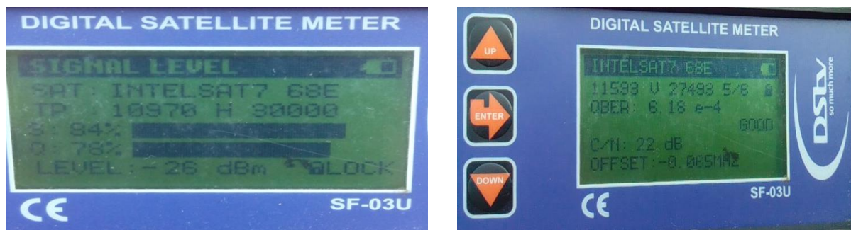
Fig 4.1 Received signal level and BER respectively for a 60cm antenna under clear weather.
