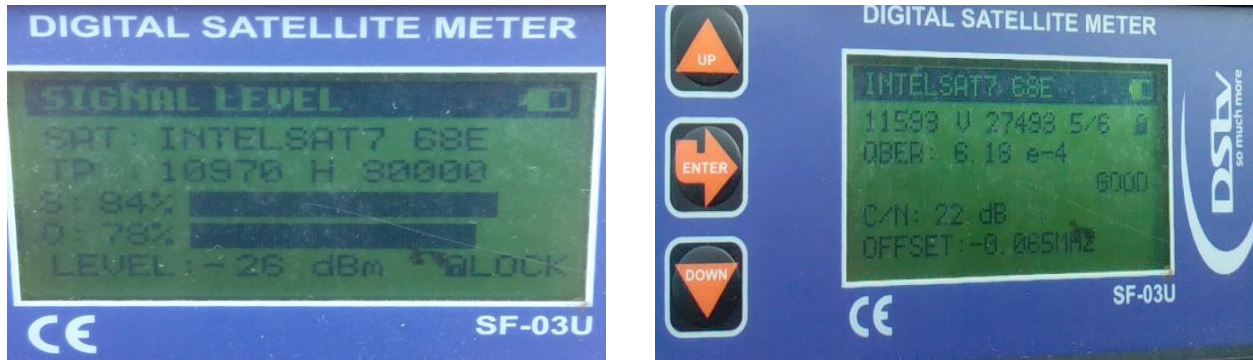
Fig 4. Received Signal and Quality Level and BER for 90cm antenna
