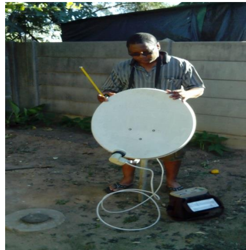
Fig 3.2 (a) Using tap water to simulate the effect of rain fade. Fig 3.2 (b) Test Preparations
