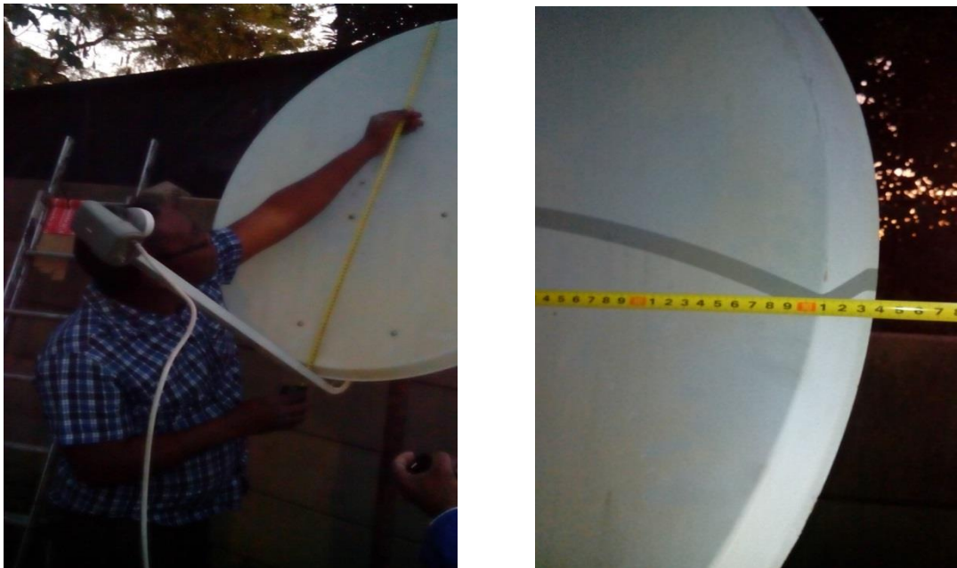
Fig 3.1 Testing setup. Measuring the actual size of the antennas
