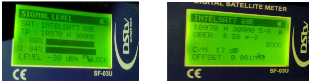
Fig 4.4 Signal quality level and BER for 90cm antenna under light rain conditions
