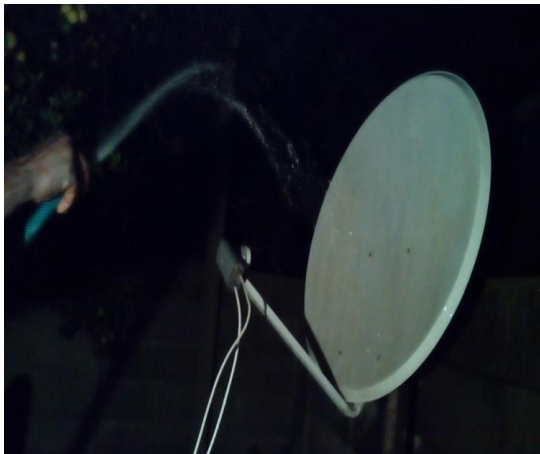
Fig 3.2 (a) Using tap water to simulate the effect of rain fade. Fig 3.2 (b) Test Preparations
