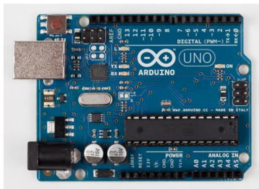
Figure 2.1: Front of the Arduino Uno Board [3]
