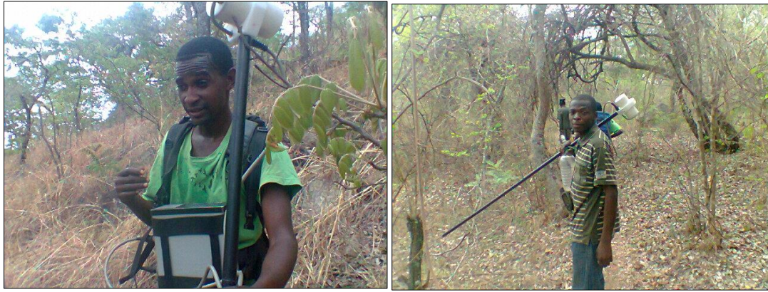
Fig 23 the magnetometer computer box unit and the sensor being used to collect readings during the Nyanda mountains survey.
